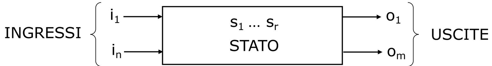
$$o_i = f_i(i_1, \dots, i_n, s_1, \dots, s_r) \quad i=1, \dots, m$$
